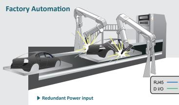
The Woodpecker 9015 Series has dual power inputs to provide a redundant system against power supply disruptions. In case of one power source failure, the other acts as a backup to remain continuous network power for critical industrial applications.
